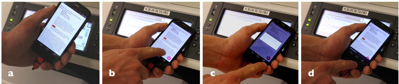
Figure 1. When a user is reading a document (a), they can tap the phone to a printer to bring up a “print” contextual charm (b). Pressing the charm spools the document to the printer (c), which prints it (d).
