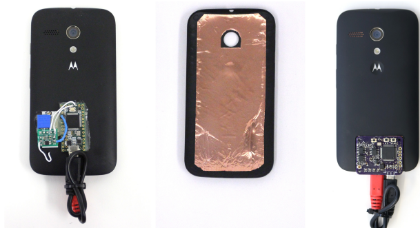
Figure 2. Our sensing hardware attached to phone. Left: original prototype. Center: copper tape antenna inlaid on rear cover. Right: final prototype with integrated PCB.
