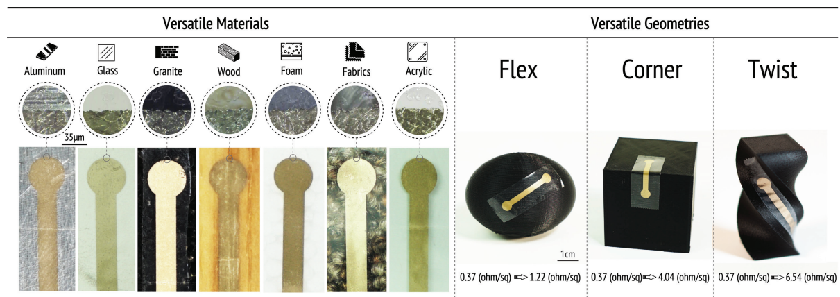
Fig. 6. Silver traces transferred onto different materials and geometries.
