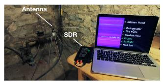
Figure 11. Sozu receiver setup deployed in a basement.
