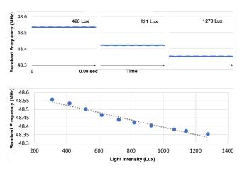
Figure 15. Top: received Sozu tag frequency at different light intensities. Bottom: mean received frequency vs. light intensity with linear regression plotted.
