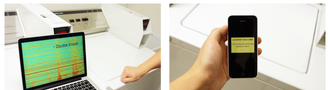
Figure 17. A user double knocks on a laundry machine to request a completion notification.
