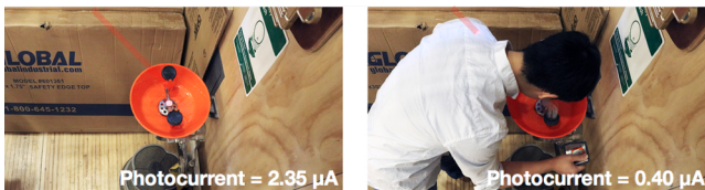
Figure 19. Tag occlusion is easily detected by measuring the reflected light intensity, and can be used to infer use.
